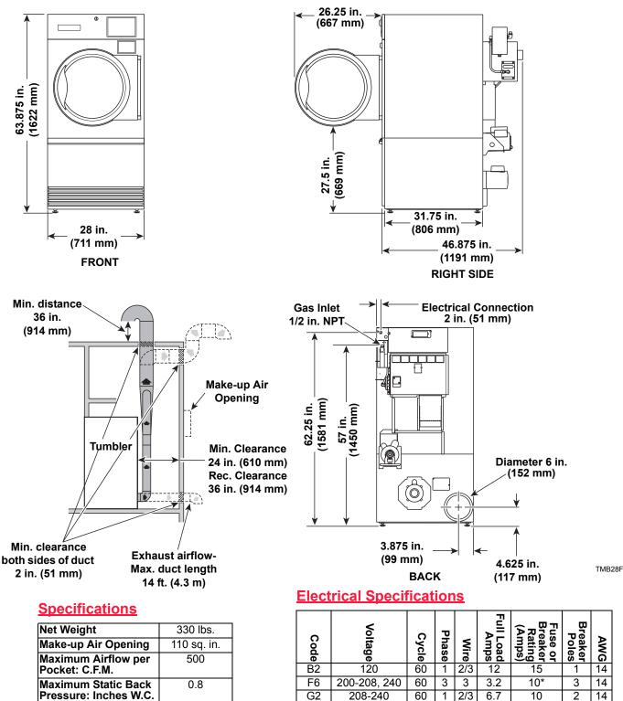
3 3 Phase machines should not have fuses, breakers only.
